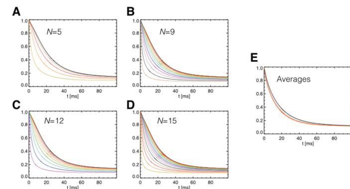
Figure 3: Simulation of the decay of  $M_z$  in the MW compartments, when starting with all  $M_{z,i}^{MW}=1$  and the other compartments all at zero, while ignoring relaxation. A-D show the individual layers for models with  $N=5,9,12$  and  $15$ ; E shows the averages over the MW compartments for the different  $N$  values.
